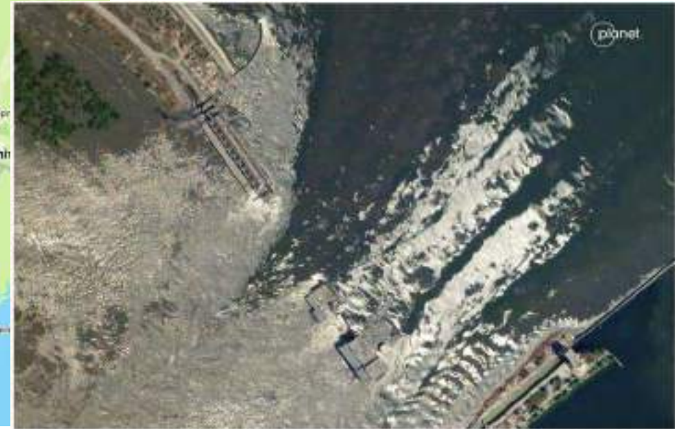
Figure 3. Satellite image shows the Nova Kakhovka dam breached (Image from Skywet courtesy of © 2023 Planet Labs PBC, available under a Creative Commons BY-NC 2.0 license at https://www.planet.com/gallery/#/post/destruction-of-the-kakhovka-dam )
